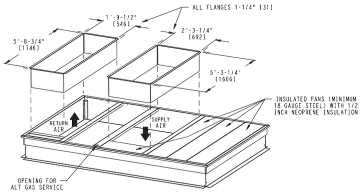
Fig. 4 - Roof Curb Dimensions - 50 TCQ-17
